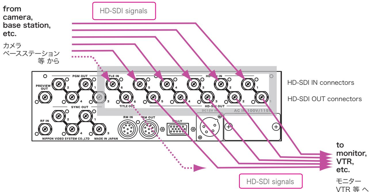
2 Connect the HD-SDI OUT 1 to 6 connectors to a monitor, a VTR, etc. with BNC cables.
