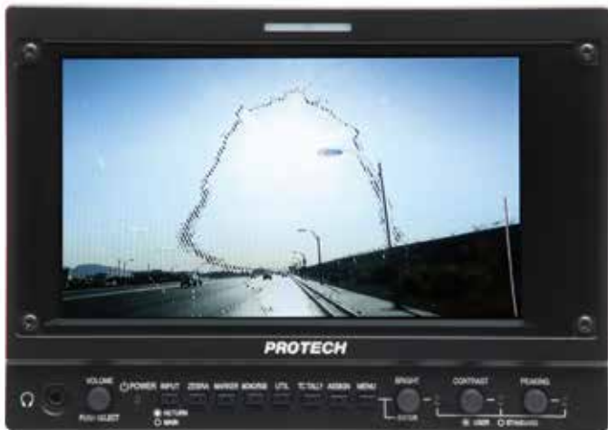
Equipped with zebra pattern that makes it easy to focus on overexposed areas
